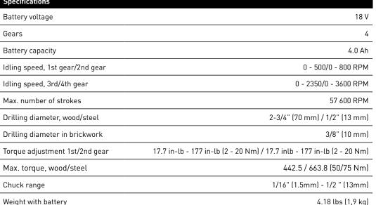
The QUADRIVE - four gears, with the right one for every application 1st gear: Demanding tightening of screws up to 3/8" (10 mm). 2nd gear: Quick driving up to 5/16" x 11-13/32" (8 x 300 mm) in size.
