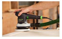
**Different strokes** The ETS 150 sanders are distinguished by their stroke size; one for intermediate, and the other for super-fine sanding.
